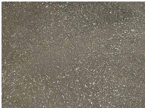
Spray pattern for bonding Pro Series AMB 2000 to the substrate "Light Spray Method"
